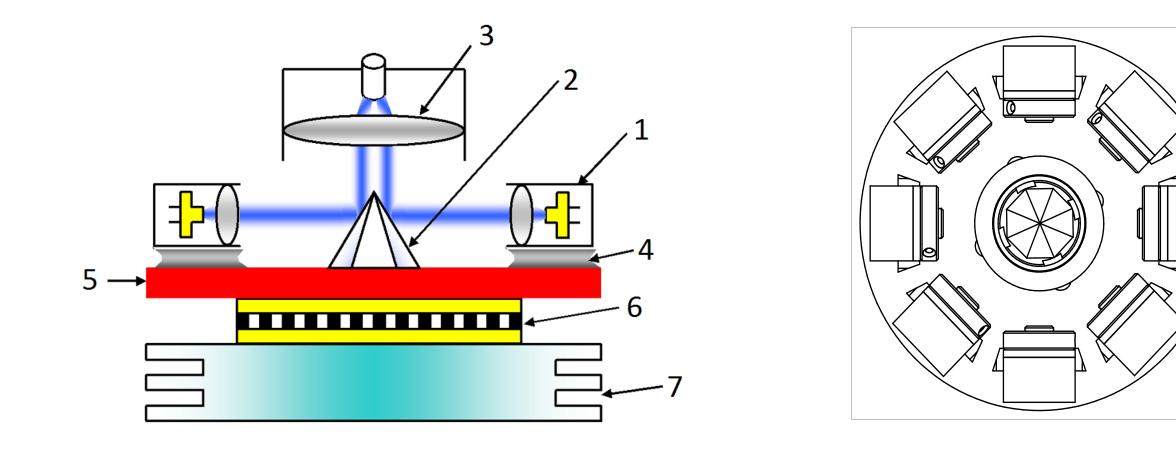
We can achieve high power monochromatic light or mix up to 8 different colors in one fiber (white light can be obtained by mixing red, green and blue) US patent US 9223123 B2
