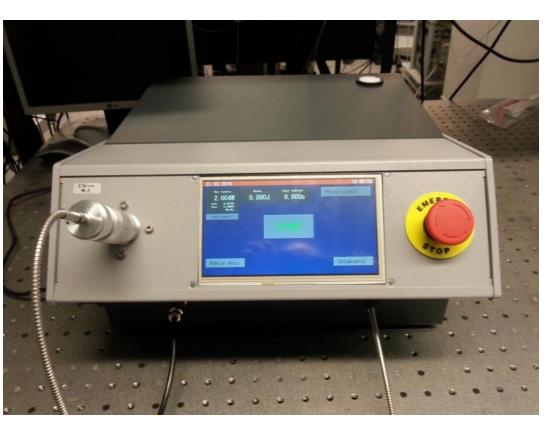
CW power achieved: 3.5W at Violet (410 nm), 50W at Blue (450 nm), 5W at Green (520 nm), 8W at Red (638 nm, with 19x1 fiber combiner). Pulsed operation from 1 ms upwards. Triple-wavelength sources: Red + Green + Blue and Red + Violet + Blue for oral PDT
